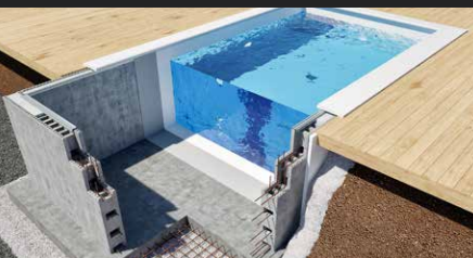
EPS/ISO blocks construction
