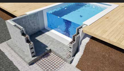
EPS/ISO blocks construction
